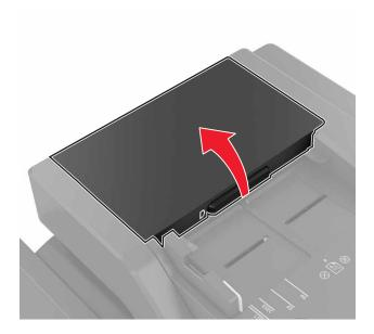
**3** Remove the ADF separator roller cover.
