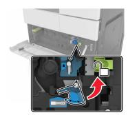
**4** Remove the photoconductor unit.
