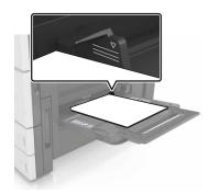
**5** From the control panel, set the paper size and paper type in the Paper menu to match the paper loaded in the feeder.
