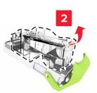
**4** Insert the new cartridge into the cartridge holder.
