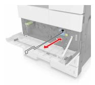
Remove the printhead wiper.
